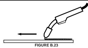
When using the GMAW process on light gauge material, weld from right to left (if you are right handed). This results in a colder weld and has less tendency for burn through.
